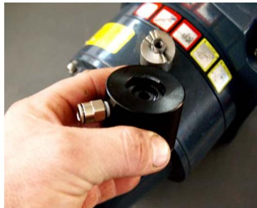
This photograph shows the freespool module removed. You can see how the
