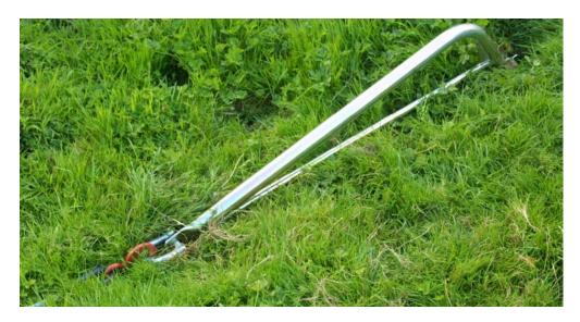
Constructed from high strength Domex steel for the blade and Cold Drawn Seamless steel for the main boom giving it very good strength but still weighing in at only 8 kgs.
